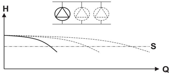
Figure 4: 1 pump in operation
