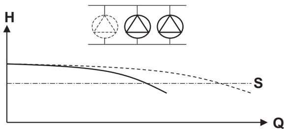
Figure 5: 2 pumps in operation
