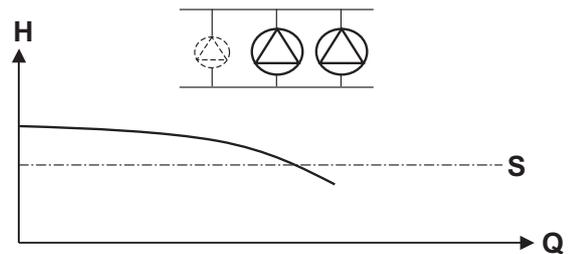
Figure 9: 2 main pumps operation
