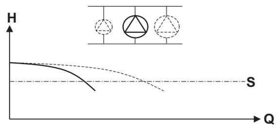
Figure 8: 1 main pump operation
