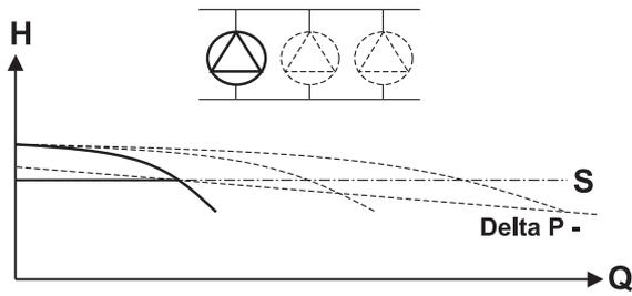
Figure 15: 1 pump operation
