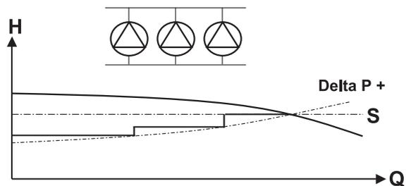
Figure 13: 3 pump operation
