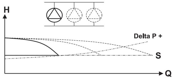
Figure 11: 1 pump operation
