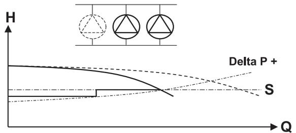
Figure 12: 2 pump operation
