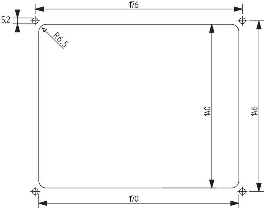
Figure 19: Build-in diagram
