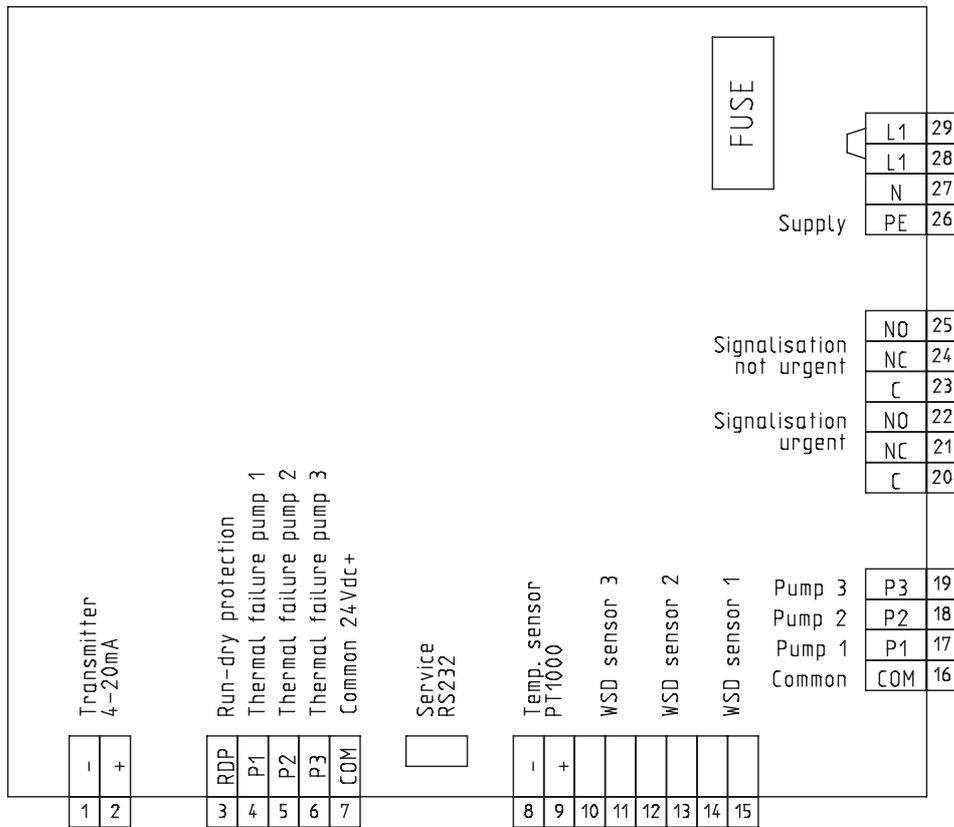
Figure 20: Electrical connections DP-Control II
